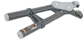
LS-TT Catenary Tensioning Tool Catenary Cable Tensioning Tool up to 880lbs with minimal effort due to the 6:1 gear drive mechanism. Integral torque gauge controls the load applied to the wire, giving consistent tension every time and optimizing the life of the wire.
